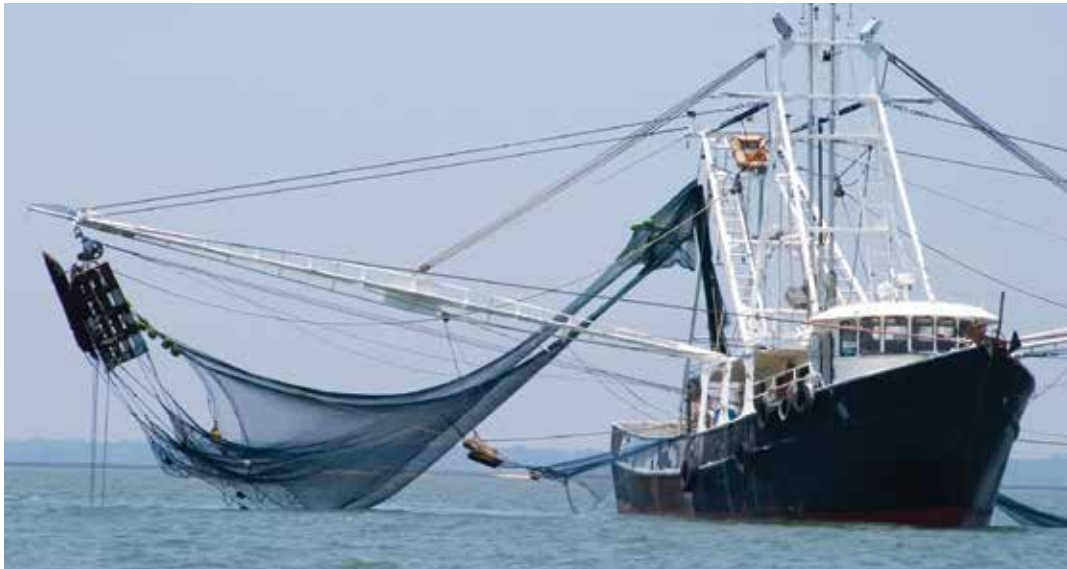
A fishing trawler empties its catch on board. The floatation devices, ropes and otter boards used to keep the mouth of the net open are clearly visible.
